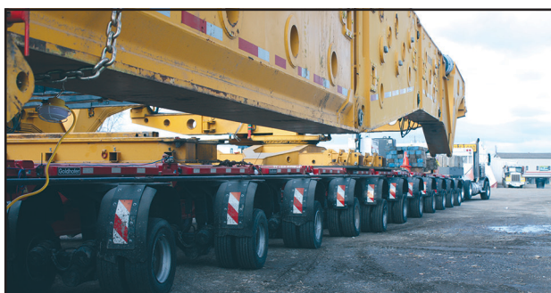
Part of the 96 wheels on the mega load transported by OxBo Transport Solutions of Scappoose, Oregon. Photo Credit: Nancy Marks
