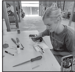
Maddie Korthas using a kitchen torch to fasten bezel to band. Photo Credits: Dee Gannon
